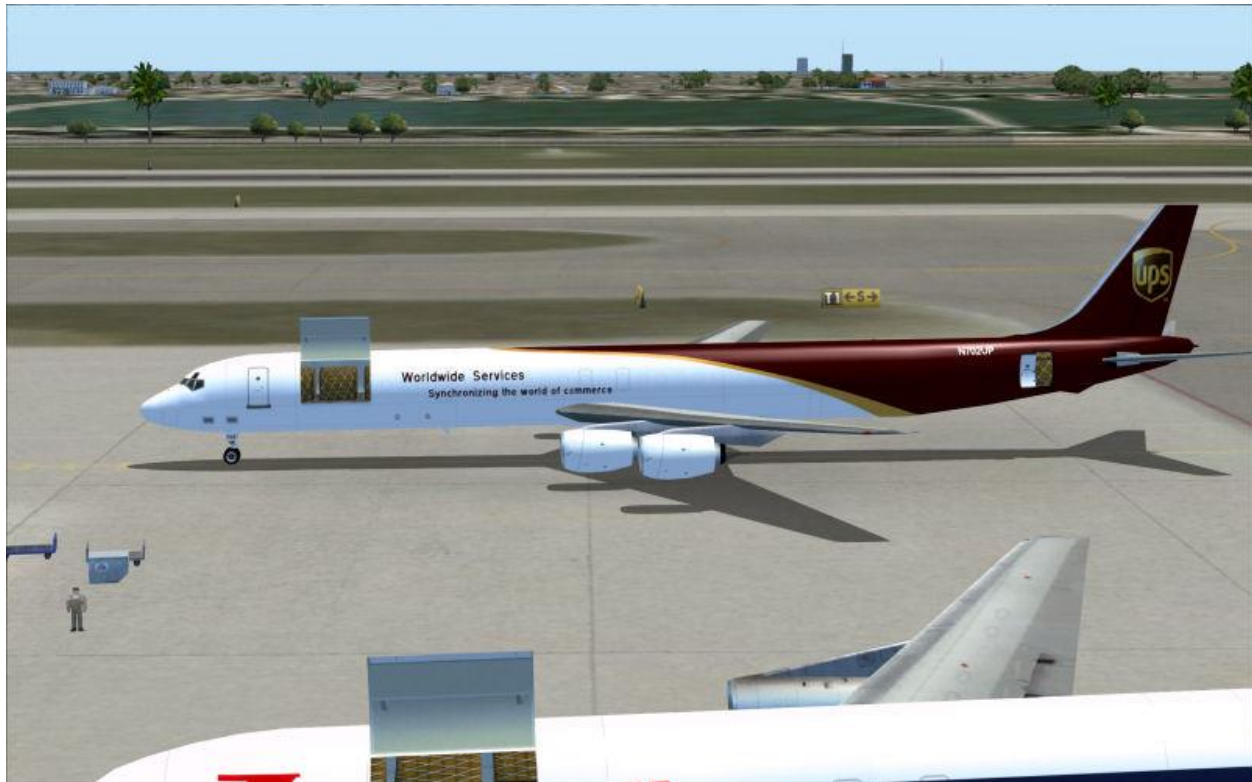
DC-8-71F showing opening main cargo deck door and service door
